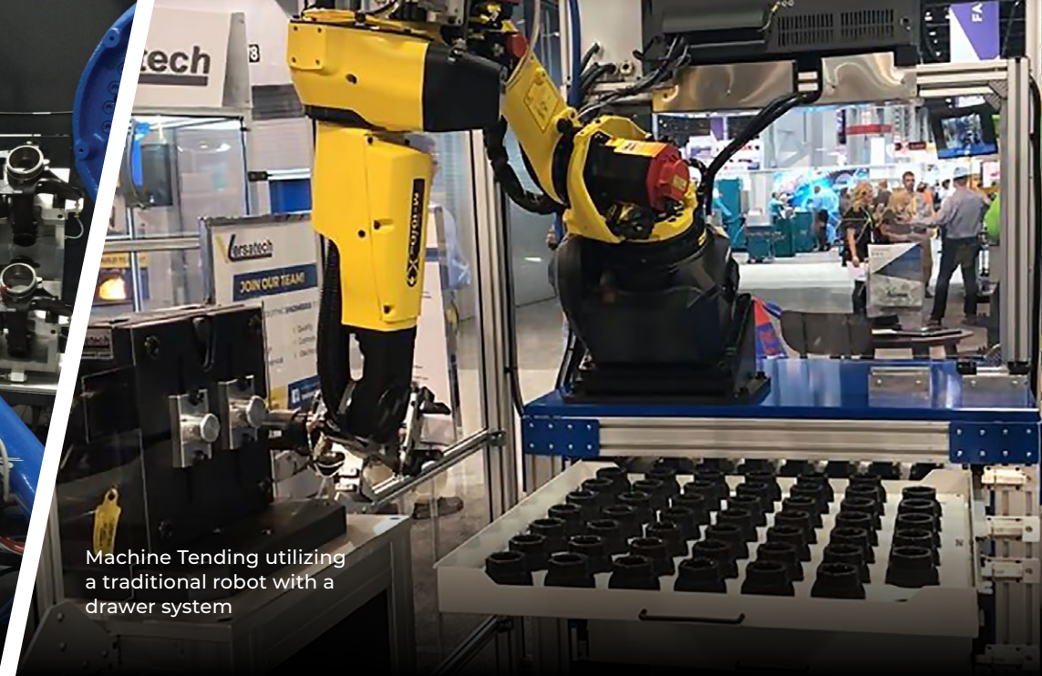
Automotive Component Machine Tending Cell utilizing a traditional robot with integrated inspection.
