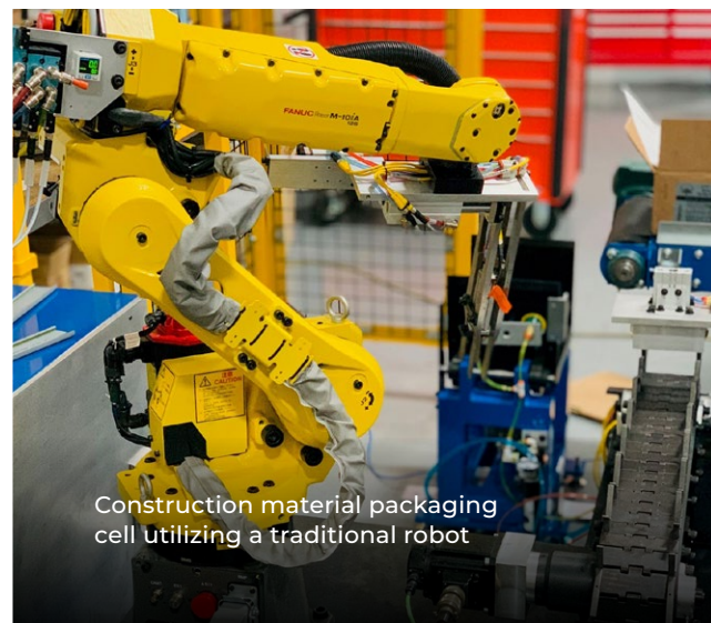
Flexible conduit packaging & palletizing cell using a traditional robot to pick a coil of conduit, load carton, close & staple carton, and palletize the finished carton
