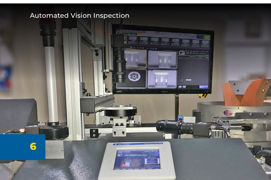
Transmission Component assembly Cell – SCARA robots utilizing a dial indexer with laser and vision inspection stations
